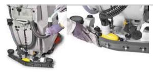
To ensure a perfect dry surface, the suction hose and the squeegee rubber blades must be cleaned at the end of any cleaning operation. The squeegee can be lifted to quickly clean the rubber blades.
