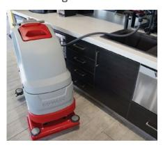
The hose for the solution tank filling can be connected directly to any water tap, giving the operator more mobility.
